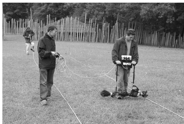
Steve Yerka (right), Yang Nan (left), and Gerald Schroedl (in background) conducting soil resistivity survey at Town Creek.
