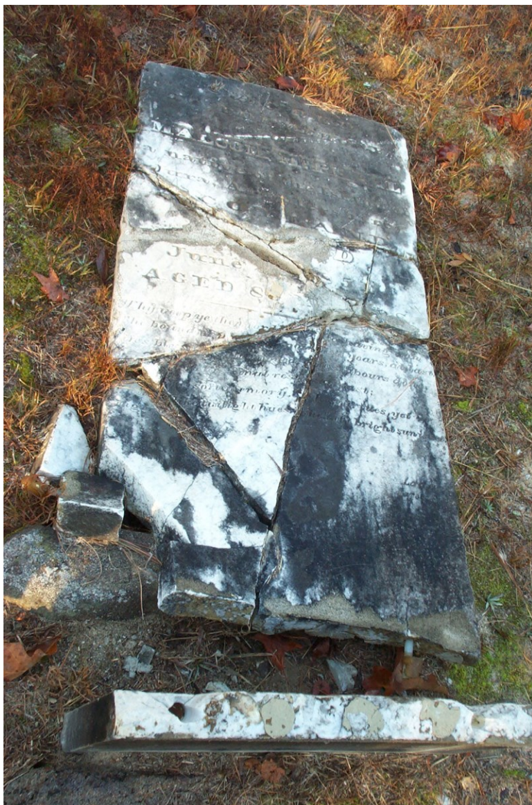
Figure 14. Example of failed pins on marker repaired in 1997.
