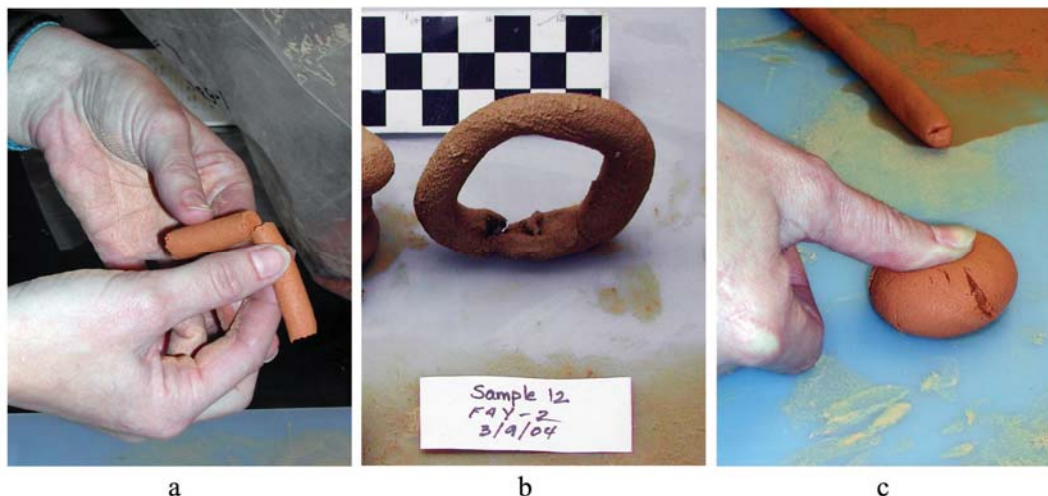
Figure 4.10. Laboratory performance tests to evaluate workability: (a) coil test; (b) loop test; and (c) ball test.
