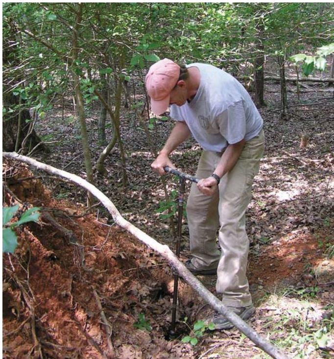
Figure 4.2. Joe Herbert using a bucket auger to collect an upland clay sample from a tree fall.
