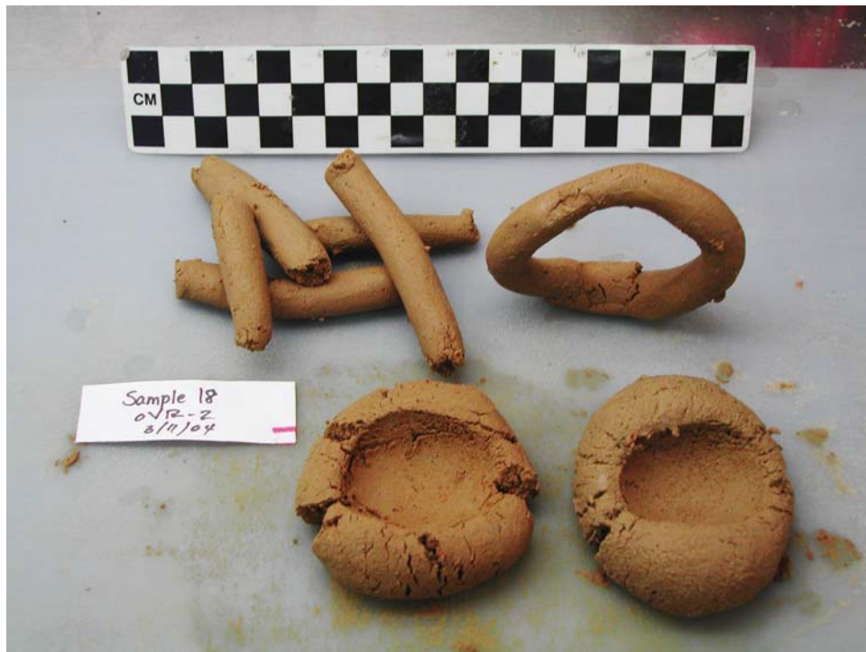
Figure 4.11. A lean sample (FBR018). Note the broken coil (upper left), sagging loop (upper right), and deeply cracked ball (bottom).
