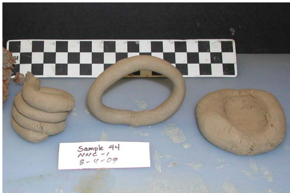
Figure 4.13. A moderately lean sample (FBR044). Note the cracked coil (left), sagging loop (middle), and cracked ball (right).
