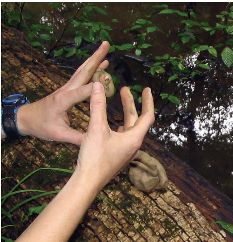
Figure 4.1. “Coil” test to evaluate plasticity.
